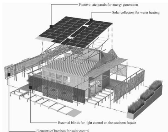
Fig. 5: Global view of the Ekó House prototype
