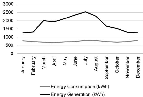
Fig. 7: Simulation of Annual Energy Balance for the Ekó House Prototype
