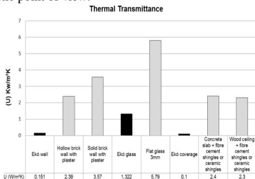
Fig. 6: Thermal transmittance of materials in the Brazilian construction industry
