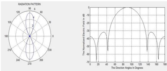
**Fig 4:- optimized Radiation pattern using Genetic Algorithm**
