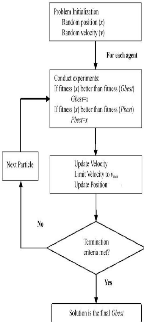
Fig 2 Particle swarm optimization flow chart
