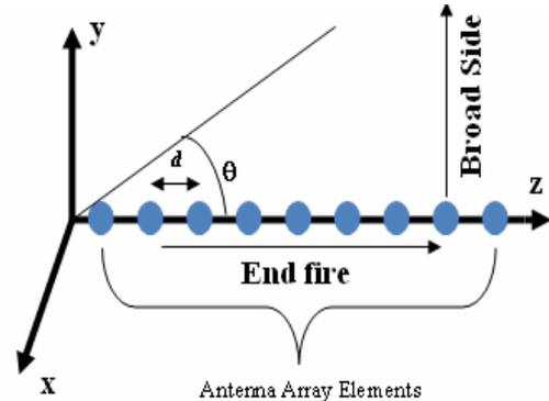
Fig:1 Uniform Antenna Array
