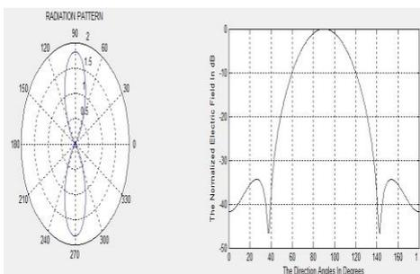
**Fig 5:- optimized Radiation pattern using PSO**
