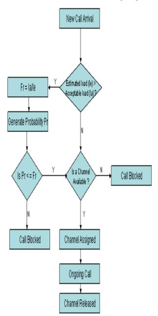
Fig. 2. Flow Chart for CAC Algorithm [3].
