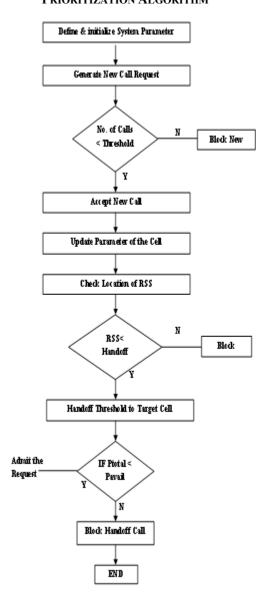
Fig. 3. Flow Chart for CAC Handoff Prioritization Algorithm
