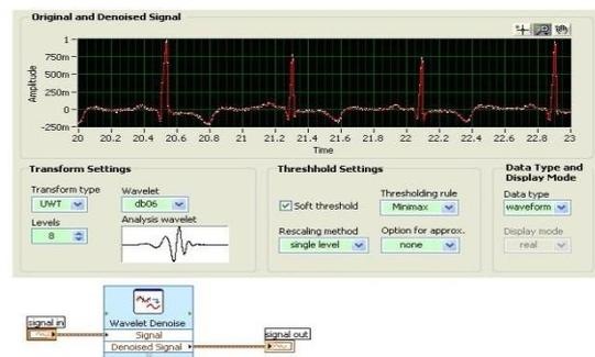
**Fig 5 Removing Wideband Noises from an ECG Signal by Applying the UWT**
