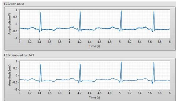
**Fig 6 ECG Signals Before and After UWT**
