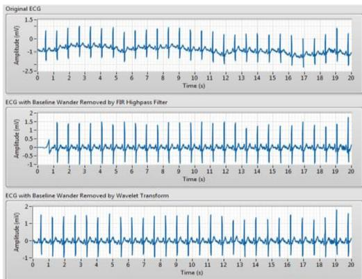
**Fig 4 Comparing the Digital Filter-Based and Wavelet Transform-Based Approaches**
