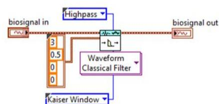
Fig 2. Designing and Using a High Pass Filter to Remove Baseline Wandering
