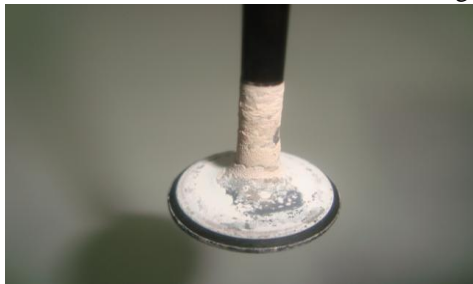
Fig 12: Eatonite Valve After Complete the Test
