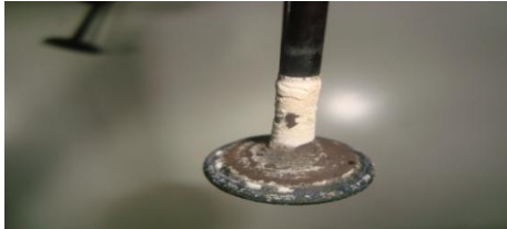
Fig 9: STELLITE Valve After Complete the Test
