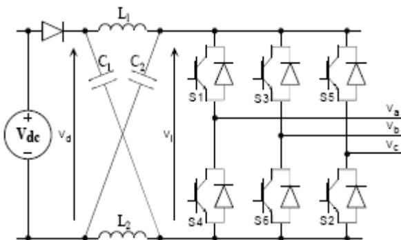
Fig 3 Three Phase Bridge ZSI Using Igbts
