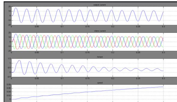
Fig 14 Simulation Results for Z-Source Current Type inverter fed induction motor drive with fuzzy controller.
