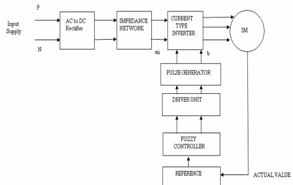
Fig 1 Block Diagram of the Z-Source Current Type Inverter
