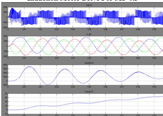
Fig 12. Boosted Outputs of Z-Source Current Type Inverter Fed Induction Motor Drive for MI=0.7.
