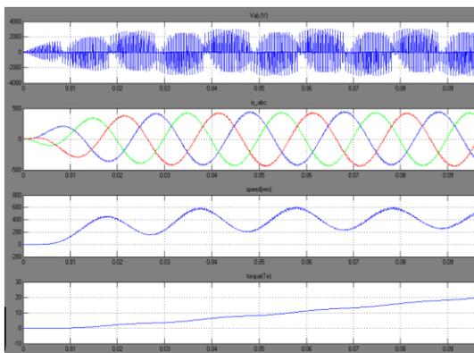
Fig 11 Buck Outputs Of Z-Source Current Type Inverter Fed Induction Motor Drive For MI=0.3
