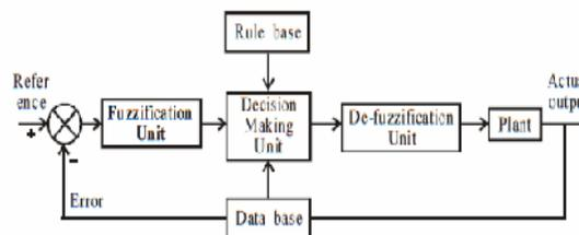
Fig 5 Internal Structure Of The Fuzzy Logic Controller.[9]
