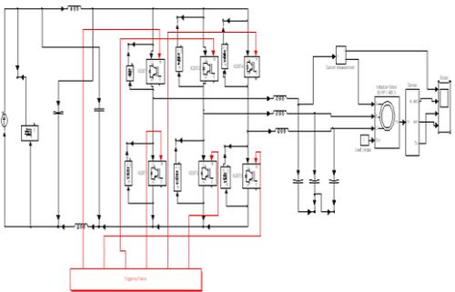
Fig 10 Simulation Diagram Of Z-Source Current Type Inverter Using MATLAB-SIMULINK.
