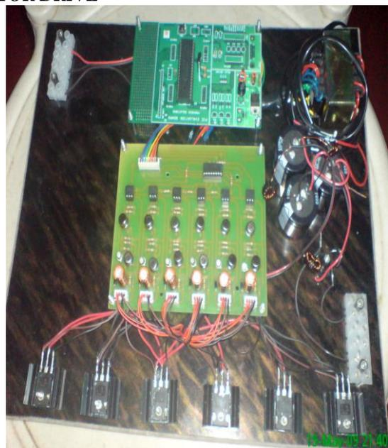
Fig 15 Hardware Prototype for Z-Source Current type Inverter fed induction motor drive
