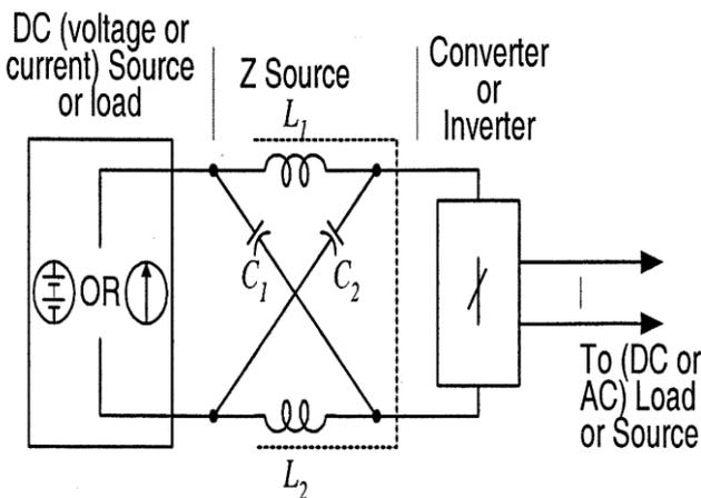
Fig.2 Z source inverter
