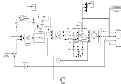
Fig 13 Simulation Diagram For Z-Source Current Type Inverter Fed Induction motor Drive Using Fuzzy Controller with Reference Value=150.
