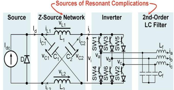
Fig 4 The topology of a Z-source current-type inverter
